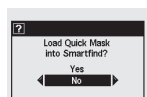
- This dialogue box (p. 37) will appear, allowing you to confirm whether or not you wish to load the QuickMask Discrimination Pattern into either the Pattern or Digital Screen.
